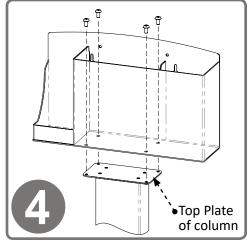
Attach the RS001-0233 Respiratory Hygiene Station to the column using (4x) screws included with stand. Tighten.
